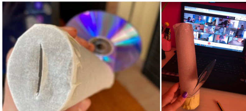
Figure 5. Students build an instrument, the spectroscope, using simple and low-cost materials and the teacher.
