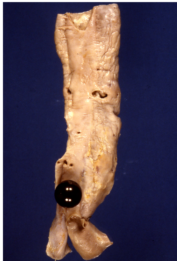
Fig. 8 Photograph shows a fatal embolism of the ball of a DeBakey-Surgitool valve after cage rupture. On gross examination, the ball was found at the aortic bifurcation.
