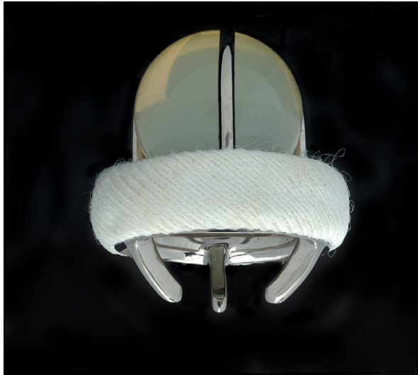
Fig. 6 Photograph shows a Smeloff-Cutter valve, with a titanium double open cage and a silicone rubber ball.
