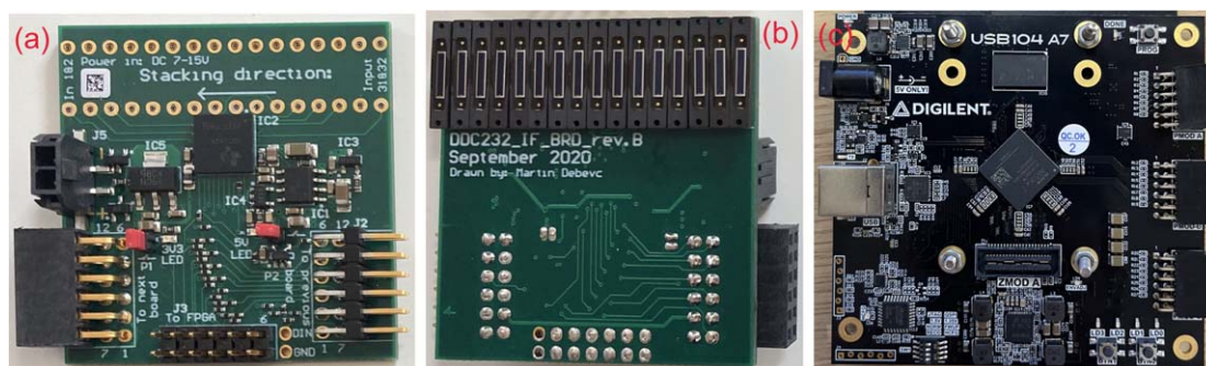
Figure 3. QuARC front-end electronics. (a) Front view of custom DDC232 circuit board. The Pmod junctions on the left and right of the board facilitate daisy-chaining while the central junction connects to the FPGA. (b) Back view of custom DDC232 circuit board showing the Hamamatsu S12915 photodiodes. (c) Digilent USB104 A7 FPGA development board. The custom DDC232 circuit is connected to one of the three available Pmod junctions on the board.
