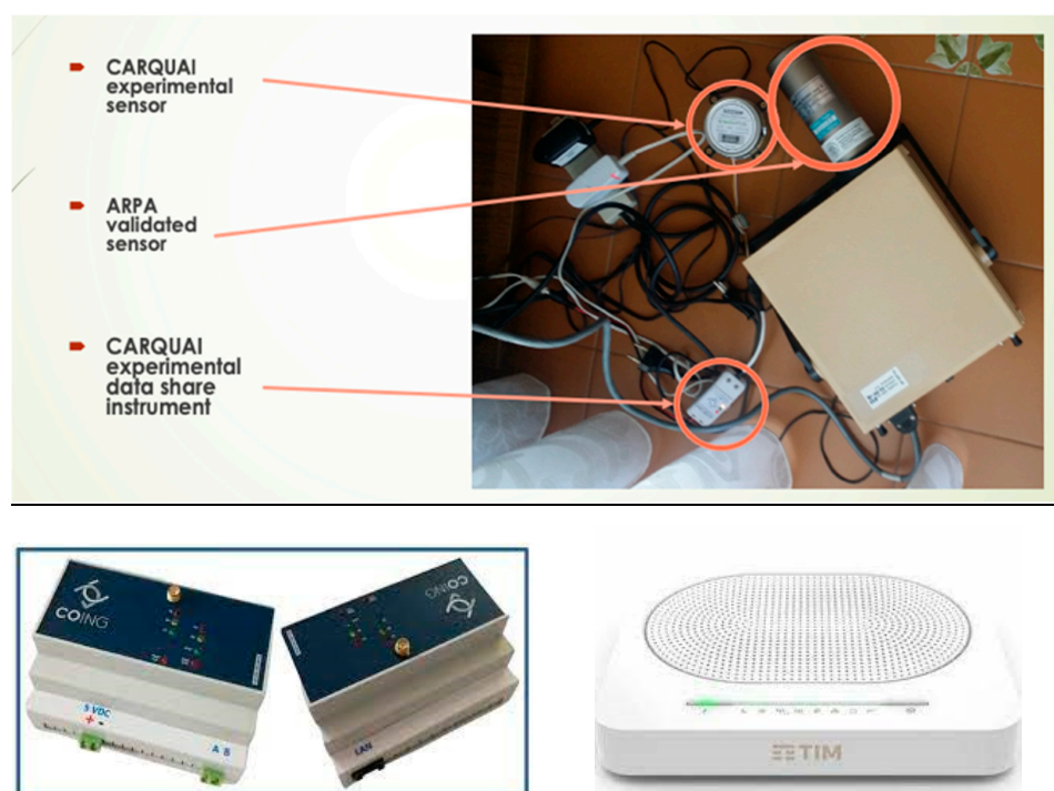
Figure 1. Experimental & validated radon detectors. Multiple data collector and web cloud system.
