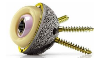
Figure 1. G7 Dual Mobility Acetabular system ® is a cup made of a titanium-alloy core, with microporous outer surface and multiple holes to improve fixation with additional screws if needed. A polar pilot hole allows for proper insertion of the chrome-cobalt definitive liner; it is coupled with a large head in highly-crosslinked polyethylene. The femoral head is compressed into it intraoperatively.
