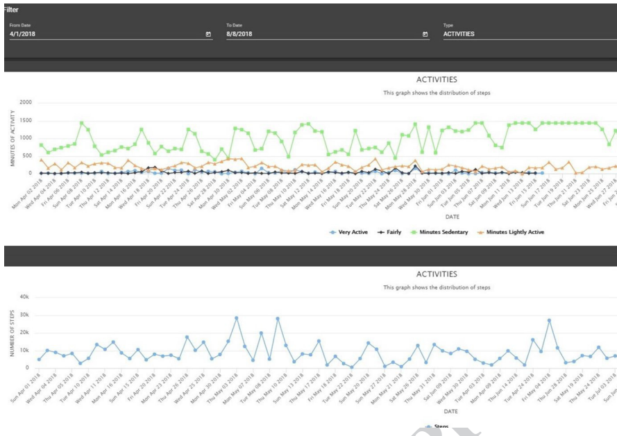
Fig. 5 Trend of users' activities over time. The first plot shows the amount of physical activity for each day, while the second shows the distribution of the steps. The time frame can be set through the date picker
