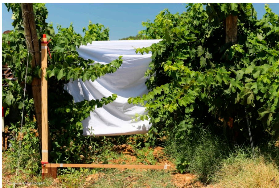
Figure 3. The wooden square angle ruler and sheet arranged on a pair of plants.
