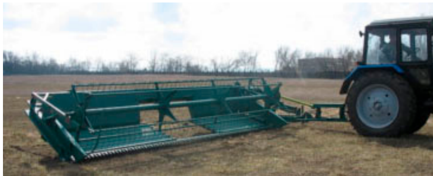
Figure 2. The asymmetric harvesting machine-and-tractor aggregate used in the test, consisting of an MTZ-80 wheeled tractor and ZhVP-6 cutter bar.
