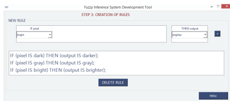
Fig. 10. Definition of fuzzy rules for the contrast enhancement using FISDeT.
