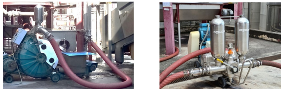
Figure 4. Pumps used for racking: peristaltic (left); piston (right).
