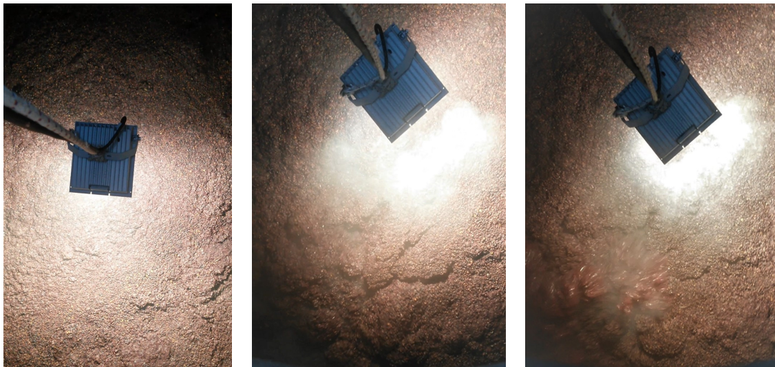
Figure 6. Grape marc cap in the process of breaking with the pneumatic system.
