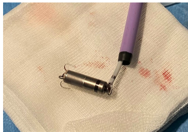
FIGURE 2 Visual inspection of Micra AV TPS after extraction. In the picture it can be observed the external structural integrity and the absence of adhesions or fibrocellular encapsulation. Micra AV TPS, Micra AV transcatheter pacing system. [Color figure can be viewed at wileyonlinelibrary.com ]
