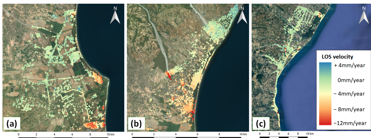
Figure 5. SPINUA measured velocities for Sibari (a), Trebisacce-Villapiana (b) and Policoro area (c).
