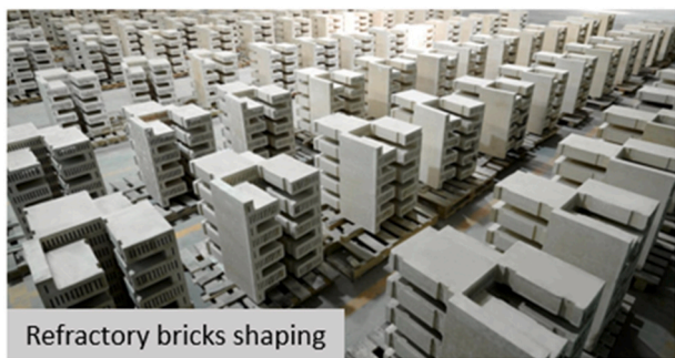
Fig. 6. Photograph of the refractory bricks manufactured and used as Rondo Energy TES media [60].
