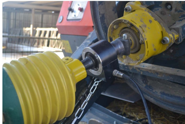
Figure 3. Contactless rotary torque transducer Datum Electronics Series PTO 420, linked to the tractor’s PTO. Source: Author’s personal archives.
