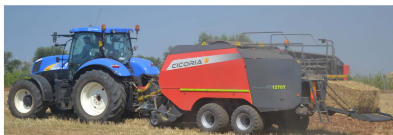
Figure 1. Big square baler (Cicoria HD 1270T) trailed by a tractor (New Holland 6090) during the tests. Source: Author’s personal archives.
