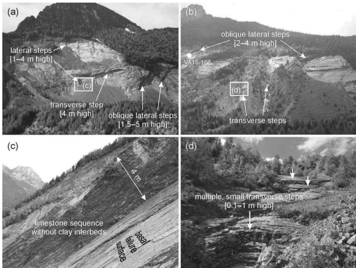
Fig. 6 300 dpi. Stepped morphology of the basal failure surface characterising (a) the eastern part and (b) the western part of the detachment surface of the Vajont landslide. (c), (d) Details of a lateral step and multiple transverse steps, respectively, showing the in-situ lithostratigraphic sequence outcropping on the failure surface (Fonzaso Fm.).
