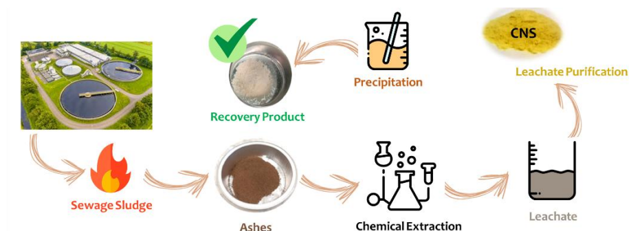
Figure 1: Leachate decontamination process to recover sustainable phosphorus.
