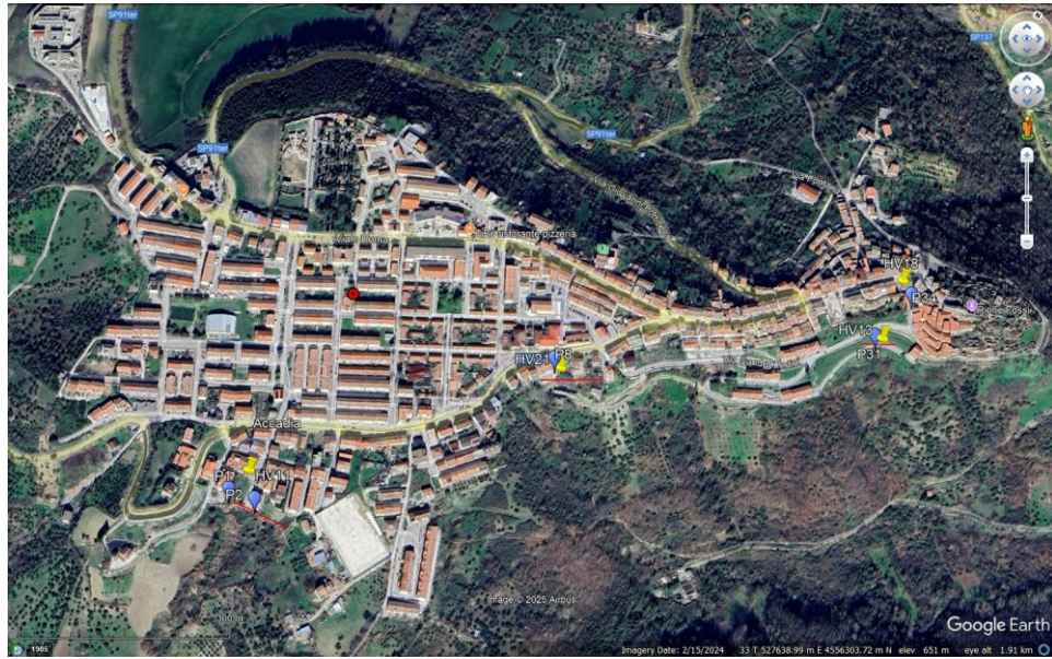
Fig. 4.22: Location of noise recording sites at Accadia (in yellow) near to boreholes (in blue) and geophysical survey profiles (red lines), whose data were used to support Rayleigh wave ellipticity curve inversion in terms of S-waves vertical velocity profile.
