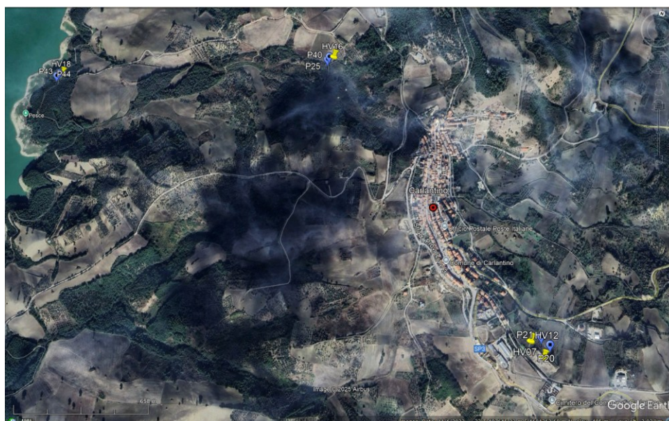
Fig. 4.32: Location of noise recording sites at Carlantino (in yellow) near to boreholes (in blue), whose data were used to support Rayleigh wave ellipticity curve inversion in terms of S -waves vertical velocity profile.
