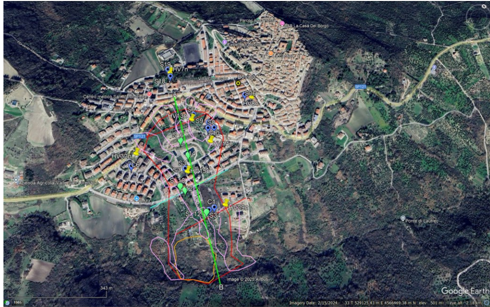
Fig. 4.26: Location at Bovino of noise recording sites (in yellow), boreholes (in blue and green, labelled with an identification code) and geophysical survey profiles (red straight lines), whose data were used to support Rayleigh wave ellipticity curve inversion in terms of S-waves vertical velocity. The boundary of the complex of the “Pianello landslide” is shown with curves of different color representing the different landslide bodies. The green straight lines represent the trace of the AB section of Fig. 4.27.
