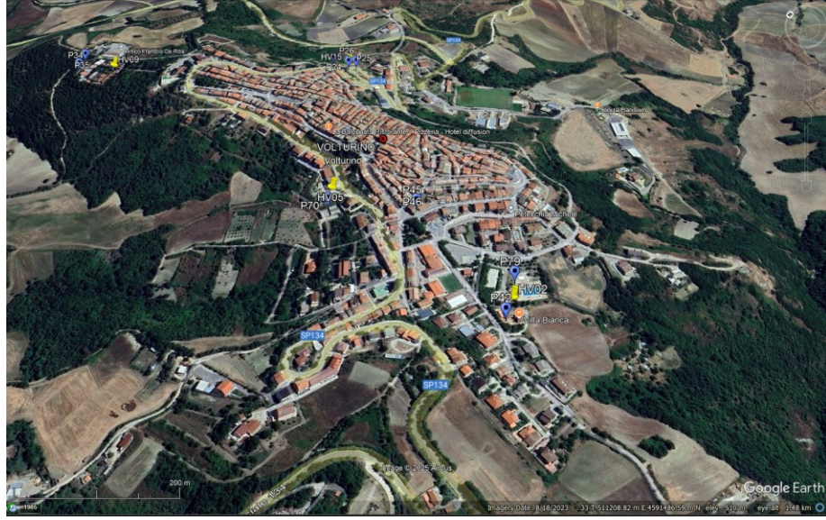
Fig. 4.36: Location of noise recording sites at Volturino (in yellow) near to boreholes (in blue), whose data were used to support Rayleigh wave ellipticity curve inversion in terms of S -waves vertical velocity profile.
