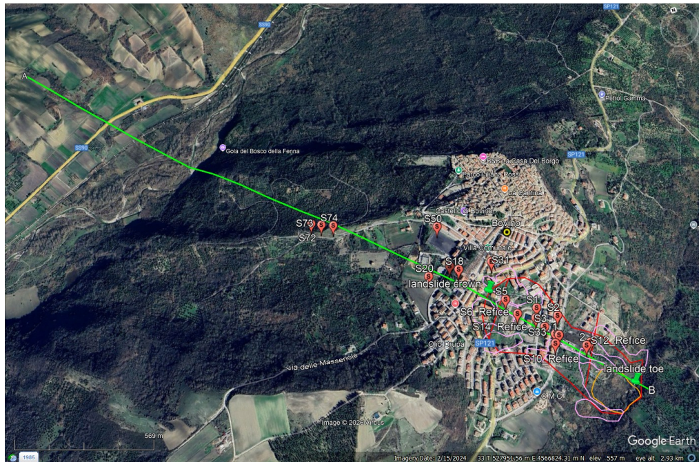
Fig. 5.12: Location of the Pianello landslide complex affecting the Bovino built-up area, with the trace (in green) of the section chosen for the 2D site response modeling. The green pointers mark the intersections with the crown and toe of the main landslide body, whose boundary is outlined in red. The red pointers indicate the position of the boreholes, while the ERT profiles are marked by red straight lines.
