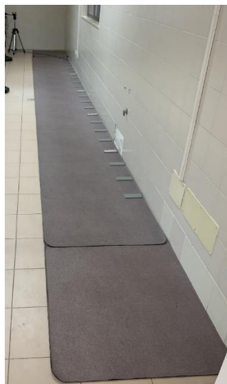
Figure 2. GAITFour ® Dog pressure-sensitive walkway used to perform this study. The PSW is equipped with encapsulated sensor pads available along the entire length of the mat. On each side of the PSW, cameras are positioned at a height of 50 cm. To identify the start and end points of the walk, an inactive mat was placed at each end of the walkway system.
