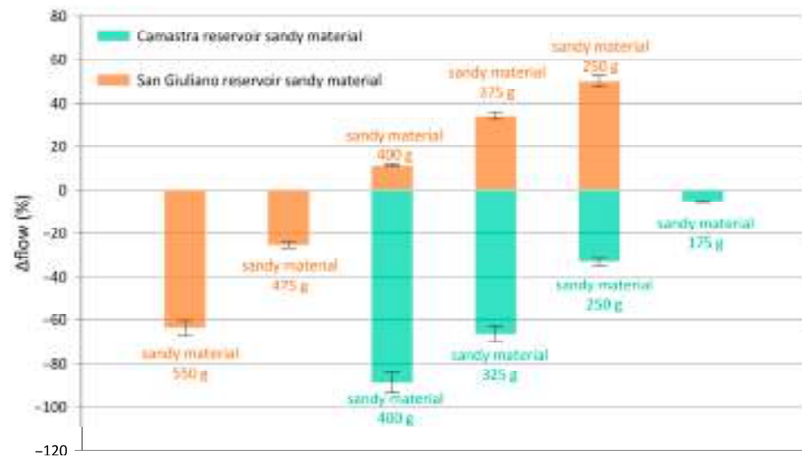
Figure 7. Comparison of relative flow values of proposed mortar obtained from sandy material.
