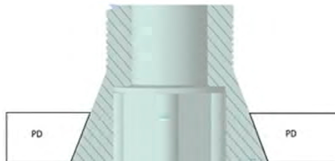
Figure 6. Cone–Morse connection at the screw–PD interface.
