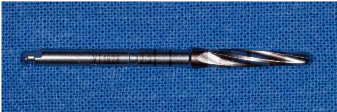
Figure 7. Third cutter with a diameter of 2.3 mm in the method “implant drilling with bone compaction instrumentation technique.”
