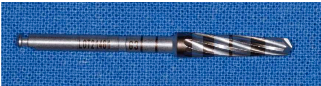
Figure 9. Fifth cutter with a diameter of 3.0 mm in the method “implant drilling with bone compaction instrumentation technique.”
