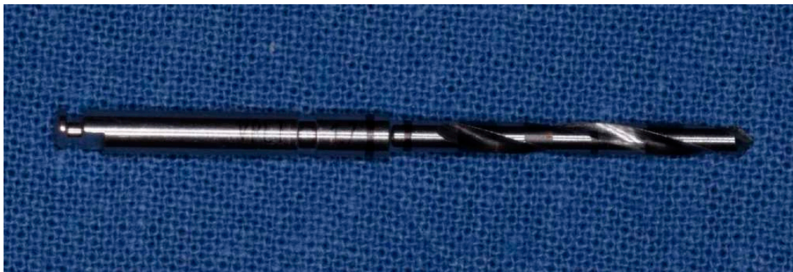
Figure 5. Initial drilling pilot cutter of the method “implant drilling with bone compaction instrumentation technique.”
