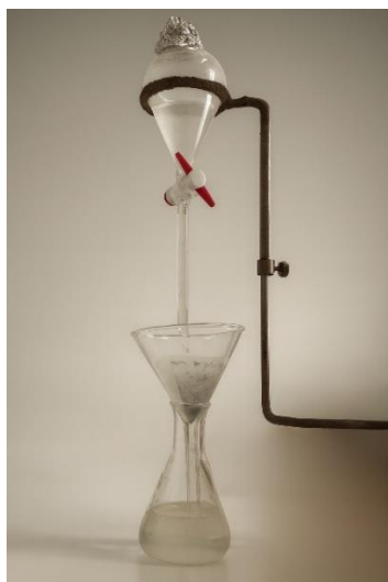
Figure 1. Continuous-flow method used for wastewater treatment with biochar.
