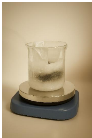
Figure 2. Batch method used for wastewater treatment with biochar.
