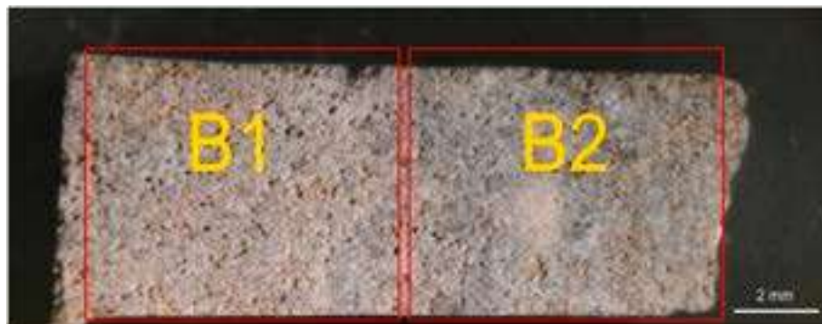
Fig. 1. Optical image of the of Al Haggounia 001 meteorite fragment. The red rectangles, named B1 and B2, represent the volumes analyzed by micro-X-ray-Computed Tomography ( \mu -CT). (For interpretation of the references to colour in this figure legend, the reader is referred to the web version of this article.)
