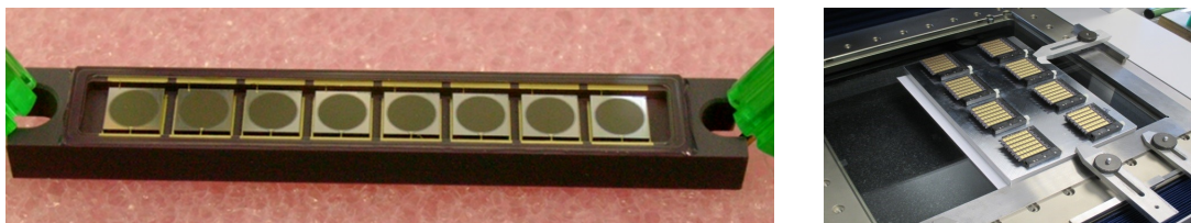
Figure 26. Left: top and side views of an eight-channel SiPM array in its ceramic package. Right: ceramic packages at the CERN Metrology Laboratory for characterization measurements.
