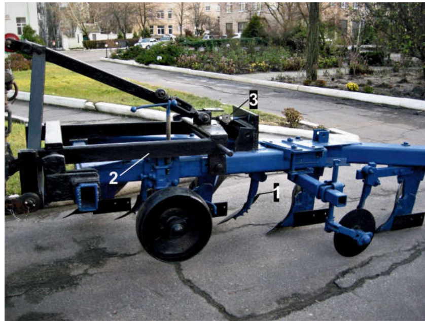
Figure 2. PLN-5-35, equipped for traction resistance measurements: 1—skimmer; 2—strain gauge frame; 3—load cell.
