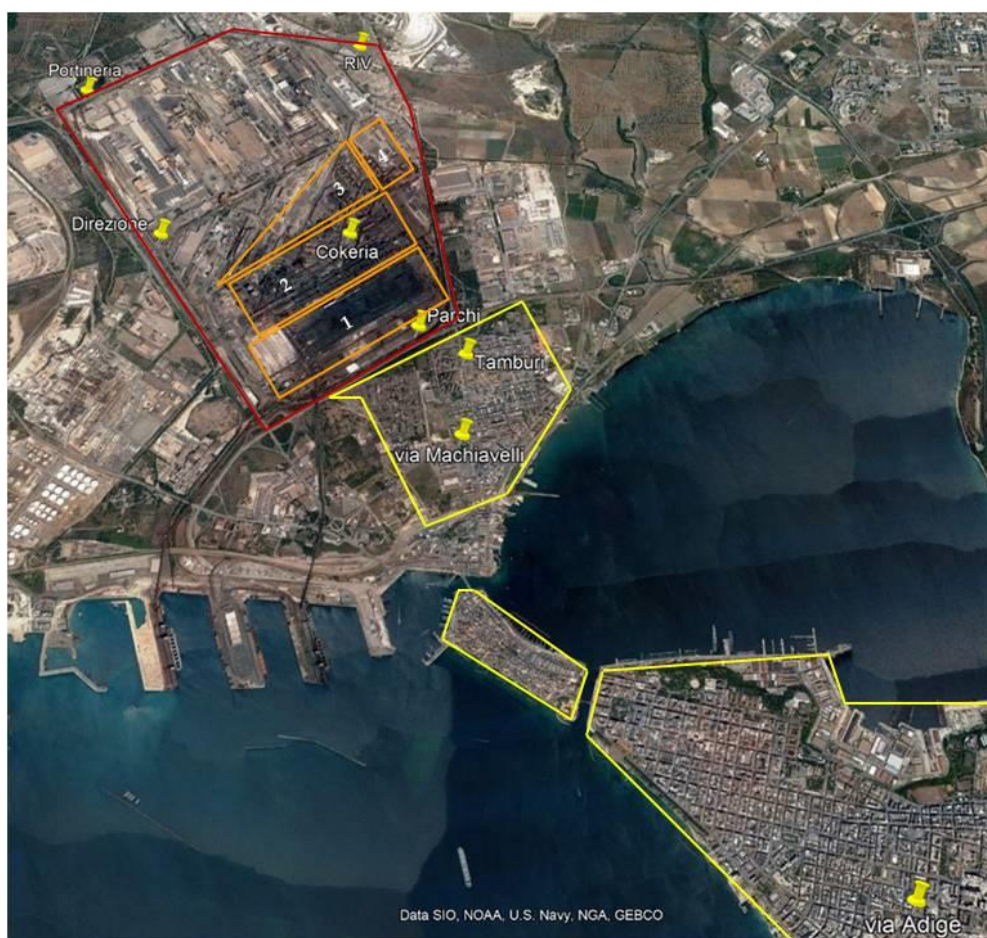
Figure 1. Position of the steel plant (delimited by the red line) with respect to the urban settlements (delimited by the yellow line). Indication of the monitoring stations inside and surrounding the steel plant and the main sectors inside the steel plant (each sector defined by the orange line). Inside the steel plant perimeter (red line): 1: mineral park; 2: coke ovens; 3: blast furnaces; 4: sintering plant.
