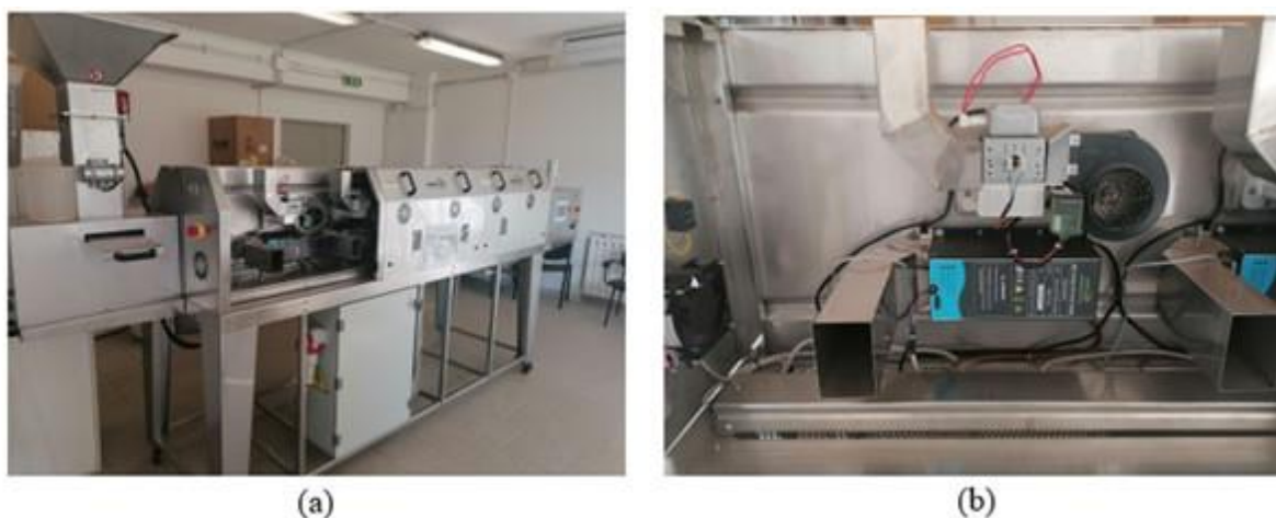
Figure 7. (a) MW-based plant prototype and (b) detail illustrating the magnetron generator, power supply, and control system.
