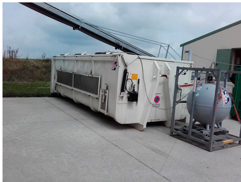
Figure 1. Container where birds are placed before treatment with CO 2 . On the left is the metal container where the chickens are placed, on the right is the CO 2 cylinder connected to the container.
