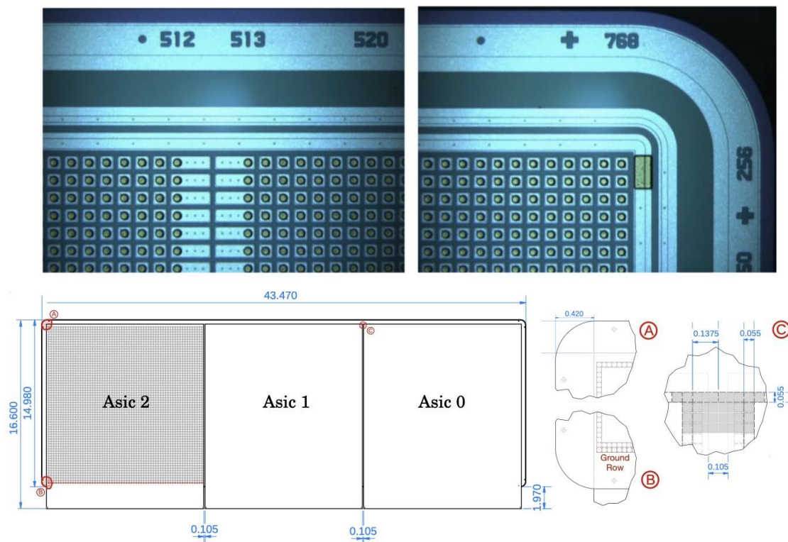
Figure 10. Top left: microscope image showing the elongated sensor pixels above the inter-ASIC region. Top right: image highlighting the ion-etched round corner of the sensor. Bottom: schematic of the sensor tile, showing the overall dimensions of the sensor and ASIC. The pixel layout is shown only under ASIC 2. There are 256 \times 256 active bonded pixels (only every fourth pixel is shown in the figure). An additional row of pixels identified in dark red provides a connection between the ASIC ground and the innermost guard ring of the sensor. Three corners, encircled in red, are shown in detail on the left (A, B, C).
