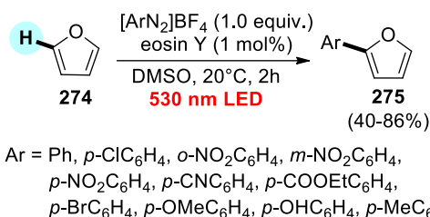
Scheme 106. Photocatalytic C2 regioselective direct C-H bond arylation of furan 274 with aryldiazonium salts, performed under 530 nm LED irradiation in the presence of eosin Y.
