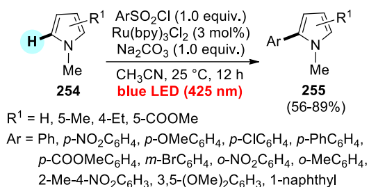
Scheme 97. Photochemical C2 regioselective direct C-H arylation of N -methylpyrroles 254 with arylsulfonyl chlorides, performed with Ru(bpy) 3 Cl 2 photocatalyst under irradiation with blue LED lamp, reported in 2016 by Natarajan et al. 303
