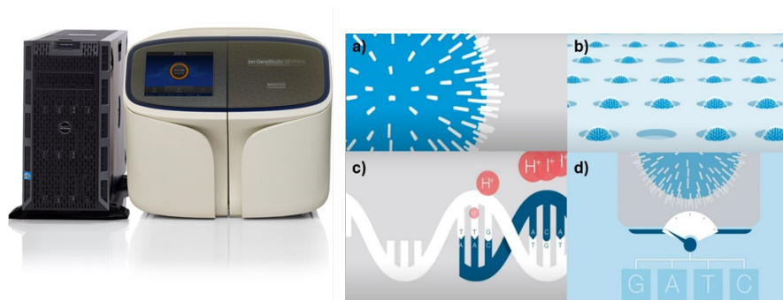
Figure 1.6.: The Ion GeneStudio™ S5 Prime System platform and the schematic representation of the Ion Torrent sequencing process, edited from Thermo Fisher website.
