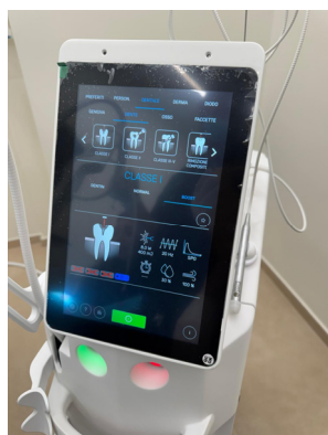
Figure 2. The screen displays specific clinical settings including power (8.0 W), frequency (20 Hz), and various treatment categories like Class I–V cavities and composite removal.
