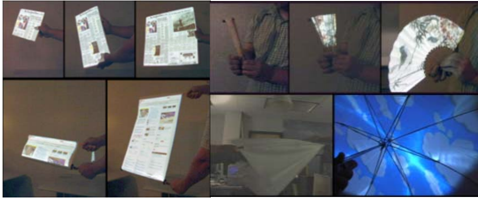
Fig. 10. Projecting the image on different surfaces, including uneven surfaces such as the interior of an umbrella or a fan [Lee et al. 2008].
