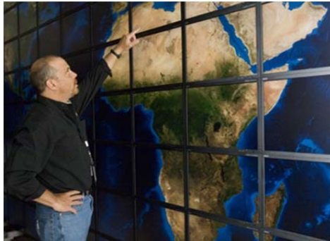
Fig. 6. The 8 \times 16 LCD panels of the Hyperwall-2 display [Bo-Wen et al. 2011].
