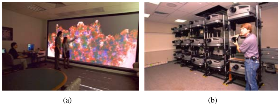
Fig. 4. The wall display (a) is built by 15 rear-projected panels (b) [Schikore et al. 2000].
