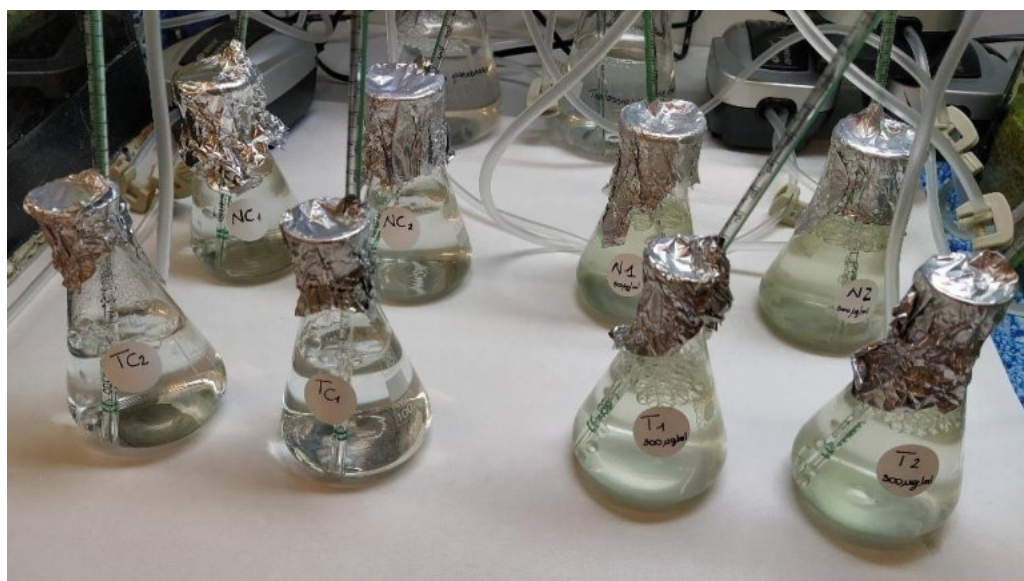
Figure 4 Toxicity tests on Nannochloropsis sp. and Tetraselmis suecica . Flasks containing cultures of the algal species Nannochloropsis sp. (back row) and T. suecica (front row) (N1-2 and T1-2 = treatments; NC1-2 and TC1-2 = controls) (photo credit: Roberta Trani).
