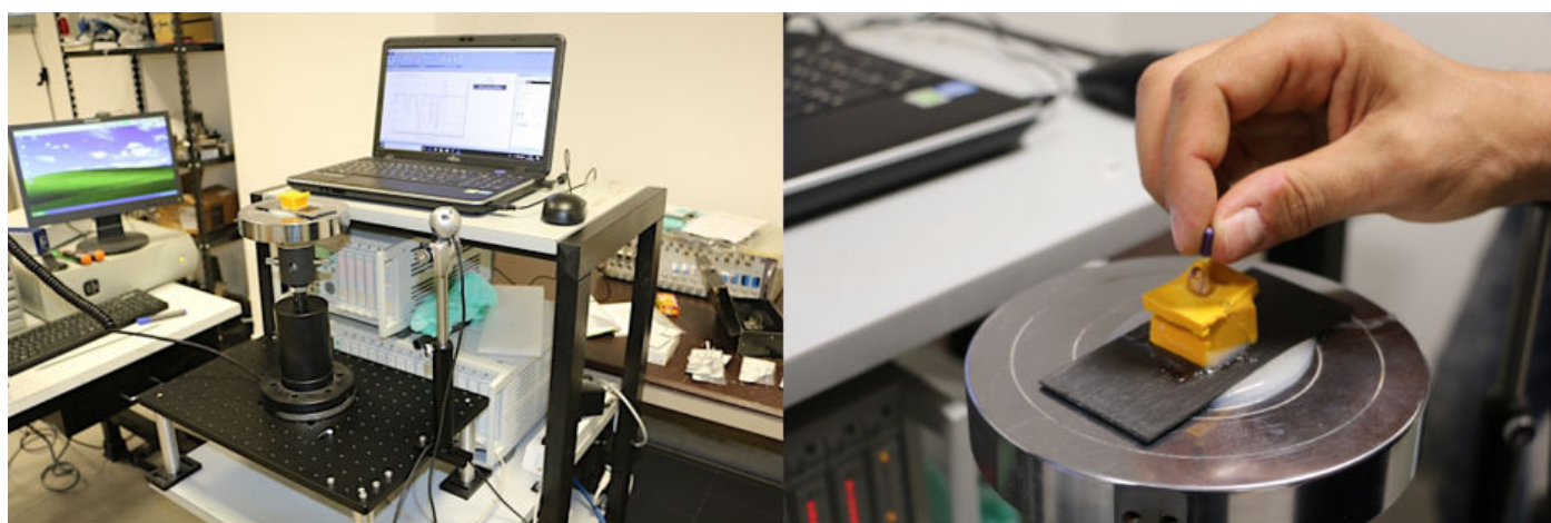
Figure 2. The testing machine. Full instrument equipment (left view) and K-file positioning (right view).
