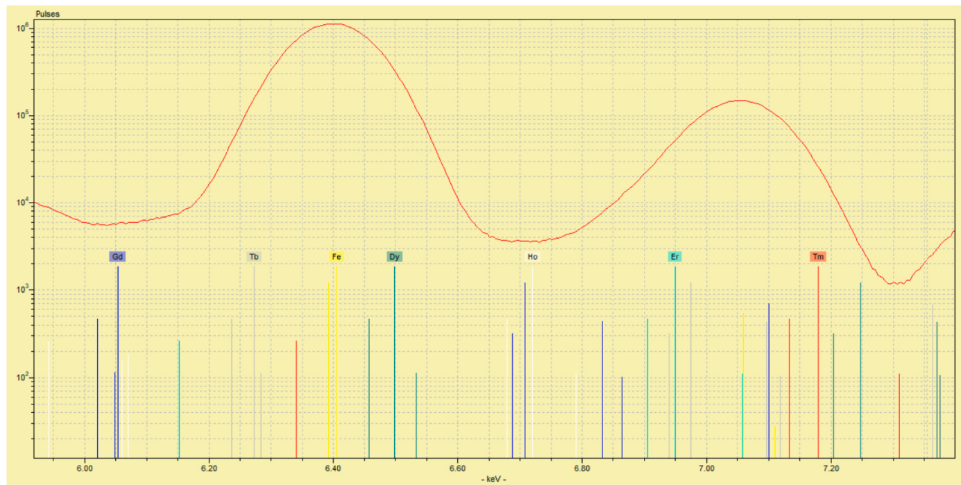
Fig. 3. The spectra of Fe after analysis of a soil sample by Picofox S2. This spectra is covering the spectra of Gd, Tb, Dy, Ho, Er, and Tm, making them impossible to be detected by this technique.
