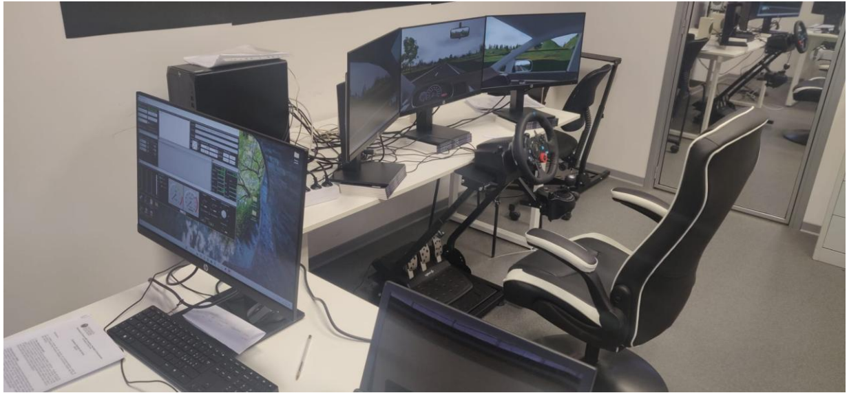
Figure 1: Our experimental setting using the CarneSoft software simulator (CarnetSoft® BV, Groningen, Netherlands). The image included three rendering monitors, a steering wheel, pedals, and a gear shift.
