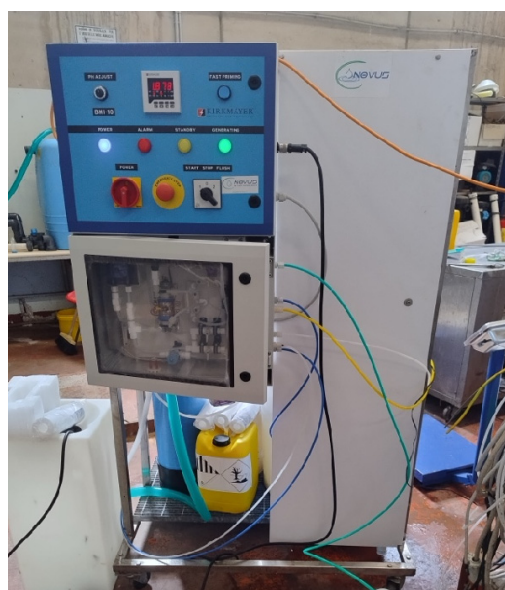
Figure 1. Generator used for AEW production.
