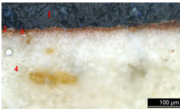
FIGURE 5 Stratigraphic section of the fragment: 1) pictorial layer; 2) gold foil; 3) bolus ; 4) preparatory layer of glue and plaster
