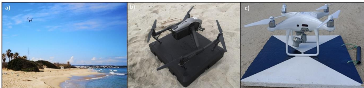
Fig. 3: a, b) Drone DJI Inspire 2 flying at Capitolo beach; c) drone DJI Phantom 4 PRO used at Torre Guaceto beach. Target used to identify GCPs is shown in (c).
